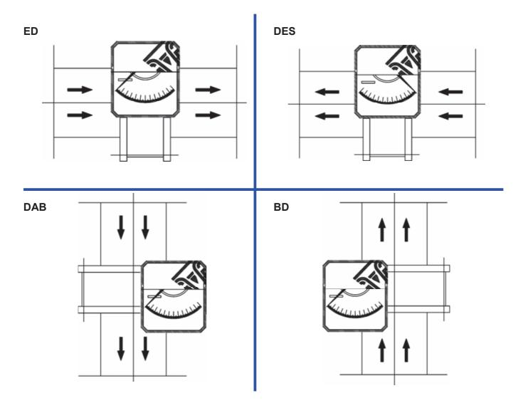
Mounting positions or flow directions different from those indicated on the scale plate can produce important reading errors or there will be no reading if the flow direction is in the opposite direction.
