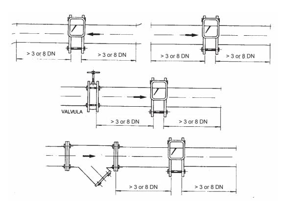
For the DP-65 series, up to DN-300, mounting must be done BETWEEN LOOSE FLANGES.
