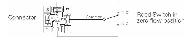
Make sure that the contact rating is not exceeded. If high loads are to be switched, use an auxiliary relay.
