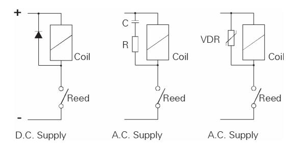
With a DC supply, a diode should be connected as shown.
