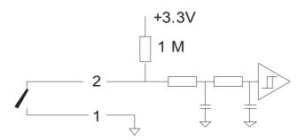
Due to the presence of a filter to avoid the effects of contact bounce, the maximum pulse frequency for the COVOL input is 300 Hz.
